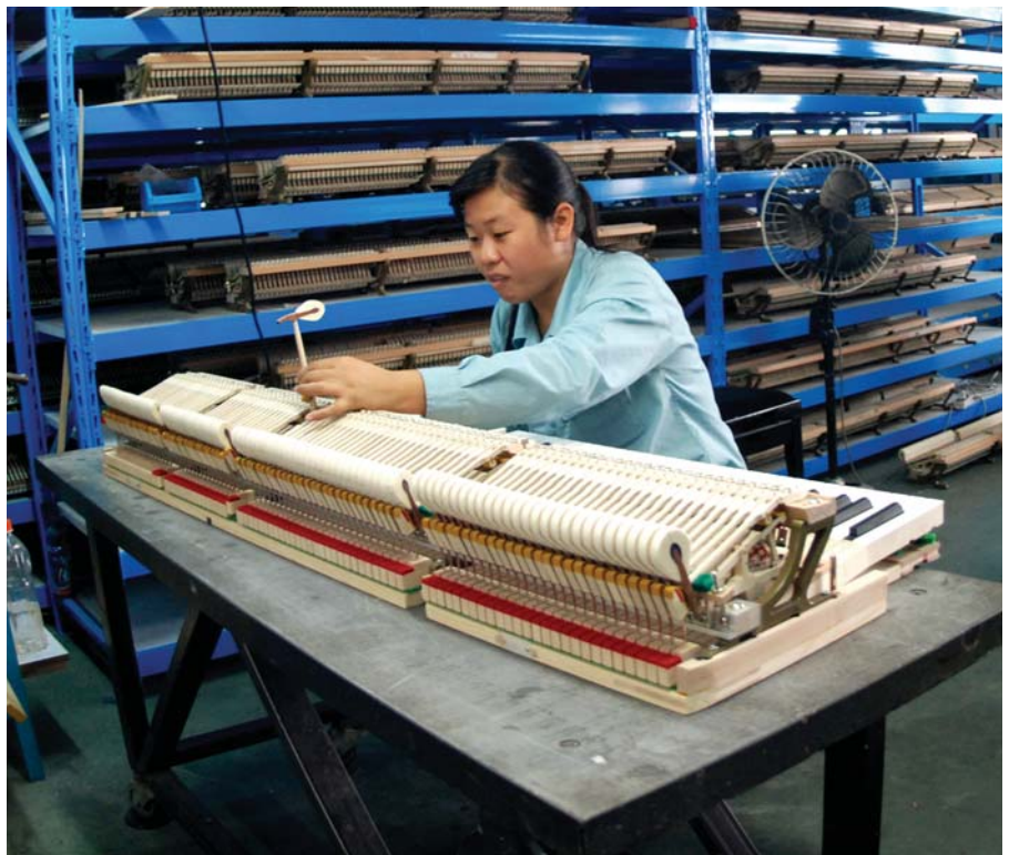
A Hailun worker installs actions at the company’s Ningbo factory. All Hailun employees are trained for at least a year before being permitted to worked on pianos destined for the market.
