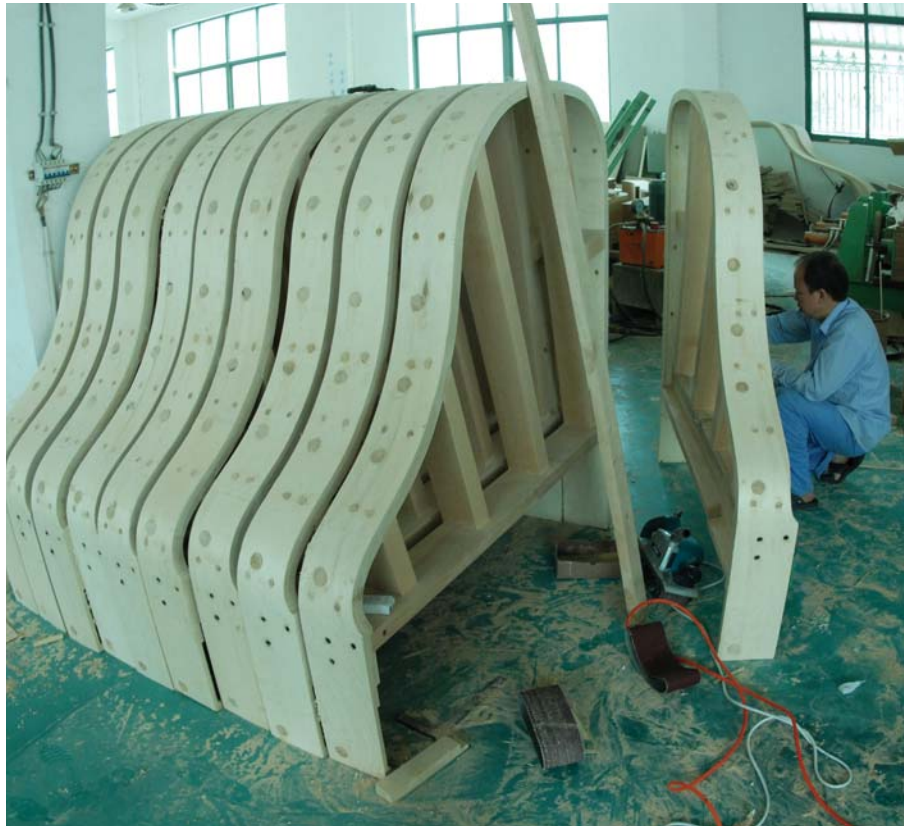
A worker sands cases at Hailun’s case factory, a separate company-owned operation outside of Beilun, a suburb of Ningbo.
