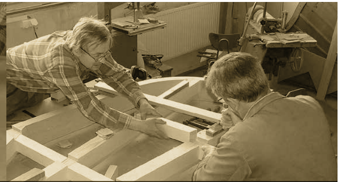
Assembly of inner frame.
